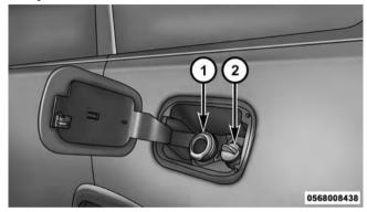
Fuel and Diesel Exhaust Fluid Fill Location
