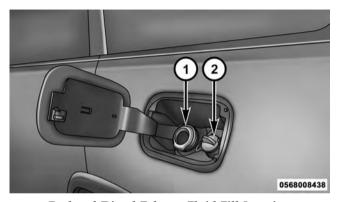
Fuel and Diesel Exhaust Fluid Fill Location
