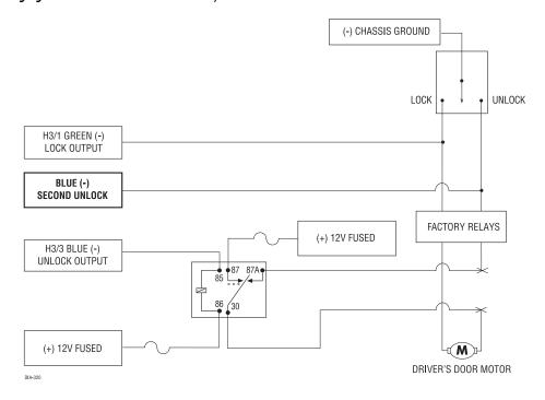
Type C (+) reversing polarity system: Wire relays as shown.
