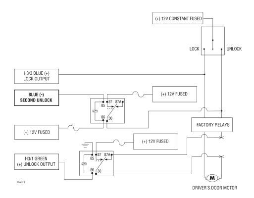
Type B (-) polarity system: Connect the BLUE H2/1 wire to the unlock wire in the vehicle and wire the relay as shown.
