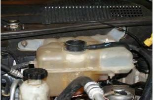
7. Disconnect the three rubber coolant lines attached to the bottle with constant tension clamps. Then pull
