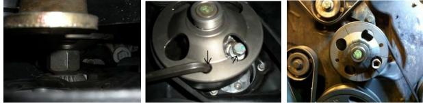
4. Relax serpentine belt tensioner (15mm bolt) by rotating clockwise and remove accessory drive belt.
