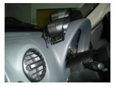
This trim piece can be popped off and lo and behold there is a connector there that contains two of the four supplies required for the gauges: Earth, and the Parking light 12V power). Anyone know what that was intended for? So by picking up two of my four leads there, and running the 12V constant power lead from the battery, I only needed to run one other which is a white lead to the good old cigar lighter lead to pick up ACC.
