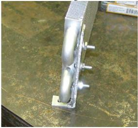
An easily fabricated aluminum L-bracket.
