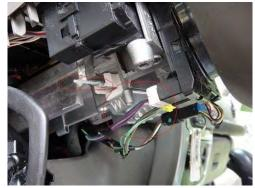
Ignition switch removed showing left end of actuator pin
