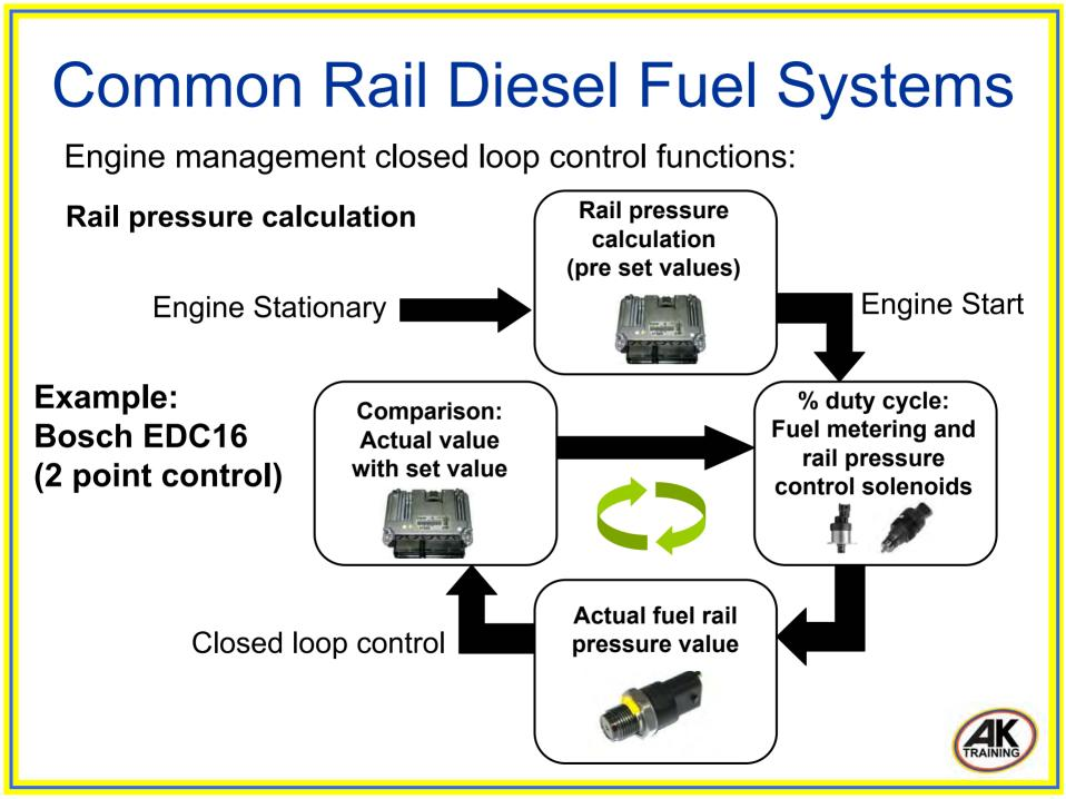
Engine management closed loop control functions:
