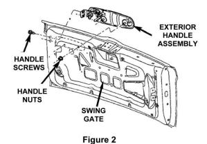
10. Remove the two (2) nuts and two (2) screws that attach the exterior handle to the swing gate and then remove the handle assembly (Figure 2).
