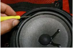
To fix this I used a handful of toothpicks to hold the detached length of foam back from the frame so that I could run glue along the surface. After the glue was applied, I removed the toothpicks and carefully made sure that the rubber ring seated itself in place against the frame.
