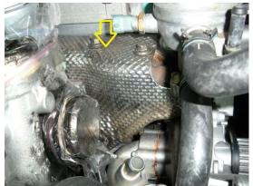
After all the coolant is drained (**NOTE - no need to do this for just timing belt job**) from the hoses you can remove the outer timing belt cover.
