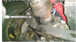
I loosened up both sides while under the car, but only remove one (this case driver side) nut, since we need the passenger side mount secured to the engine and chassis till we change the driver side, to make sure the engine will not move left or right while mounts are removed.
