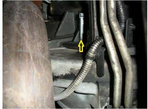
Turn the engine one (**NOTE - should do 2 turns**) full turn and reinstall the locking pins. If any of them don't go in you will have to line it back up.
