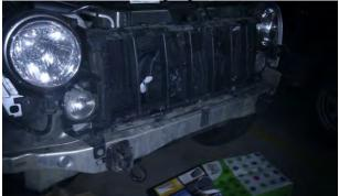
STEP 3: This is where I choose to place my cooler. I wanted the cooler to be fully exposed to the fresh air and to keep clear from blocking the radiator behind.
