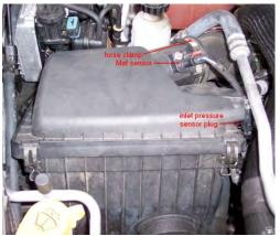
To get better access to the thermostat, we need to remove the engine air filter box. Pull up the red tab, squeeze the black section and remove the plug to the Maf sensor. Squeeze the plug to the inlet pressure sensor (you can see the catch tab lift at the front) and pull off. Loosen the hose clamp to the air intake and unclip the lid to the airbox. Remove lid and air filter element.
