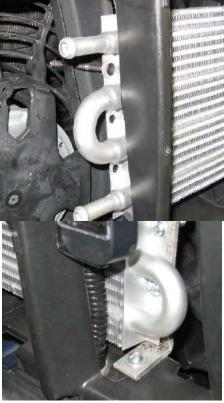
One screw in the front and one at the rear in the bracket. The setup is rock solid.
