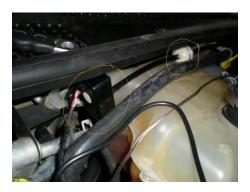
Next fitting the EGT probe (drill and tap the exhaust manifold) and consult Patracy's post on how to do this. I opted to drill it without the engine running and used the shop vac to pull stuff away from the hole, then used a magnetic screw driver to fish out the tiny bits that might have fallen into the hole.
