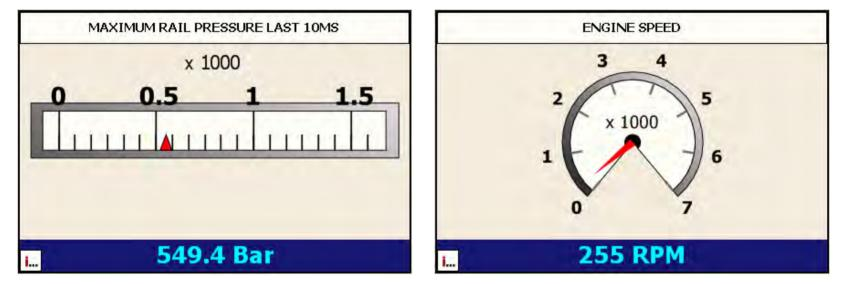
Typical minimum 'manufacturer specified' value during engine cranking:
