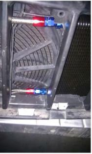
STEP 6: Trim the lower plastic in order to allow the cooler to fit. Less than an inch was enough
