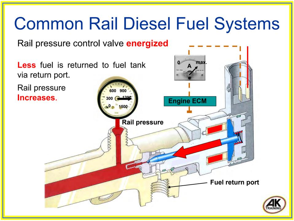
Rail pressure control valve failure symptoms and diagnosis
