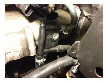
In my case I end up using 2 T connectors, so if you do break it, it's not a tragedy. Just keep in mind that one line is a hard plastic one, it won't come out from the 4 way connector and you will have to cut it and replace it with a regular hose, and that hose is connected to the fuel pump (it will add 1-2 hours to your total work time)
