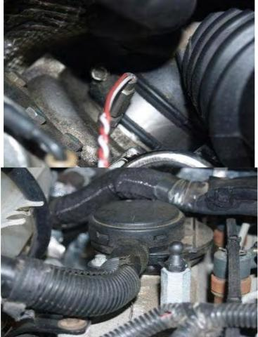
6. Remove two 10mm nuts holding the coolant bottle to the firewall.
