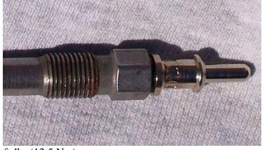
Torque the glow plugs to 9 ft-lbs (12.5 Nm).
