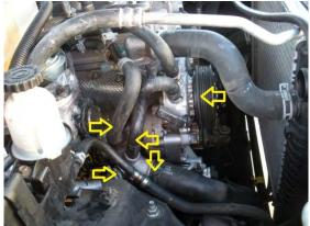
Remove (NOTE - no need to do this for just timing belt job) heat shield.
