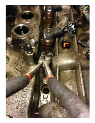
For the injector number 1, you can use a socket under the plier for a better angle.
