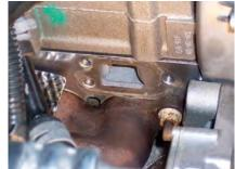
Remove 3 10mm bolts securing the thermostat to the block. All 3 can be reached with a 2.5 inch socket extention on a 6 inch wobble end socket extention. Remove the thermostat, scrape the gasket material off of the engine block and clean with acetone.
