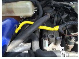
NOTE: Put your foot on the brake and put the vehicle in gear if your vibrations are worse in drive then it is your passenger side mount if it is worse in reverse it is you driver's side. The drive's side is a pain the passenger is nice and easy.
