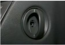
Then remove the screw in the door handle.
