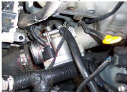
To gain access to #3 glow plug, you need to remove the intake elbow. Remove the CAC hose (8mm). Unplug the connector to the EGR Air Flow Control valve (FCV). The release tab pulls in the same direction as you need to remove the connector. Remove 4 hex (Allen) bolts (5mm) holding the FCV to the intake elbow (see next pic). You may need a tool like this to pop the bolts:
