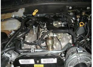
Remove (**NOTE - no real need to do this just for timing belt job**) the upper radiator hose and air hose. Cover up turbo and the intercooler so nothing gets into it. I use plastic and rubber bands so no coolant gets into it...
