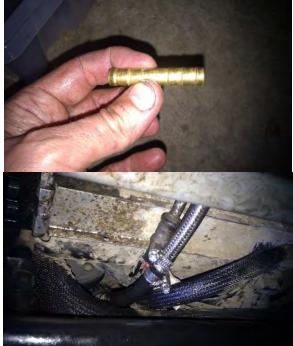
STEP 11: I decided to connect the inflow to the lower inlet of the cooler. My logic is that the oil being pushed up in the cooler has a tendency to spread in all the cooler circuit and give a better cooling effect... seems to work out well so far.
