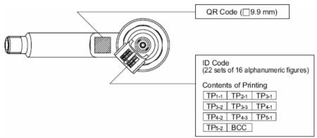
Bosch injector generation 2 IMA code for injector flow adjustment Denso injector QR (Quick Response) code
