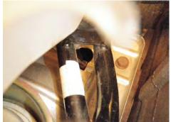
This is a shot of the oil pressure sensor which is Teed in with the factory oil pressure switch, which just happens to be 1/8" NPT. I got a male-female brass tee from Mcmaster.com
