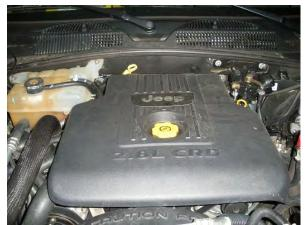
Pull straight up on the engine cover and remove it...
