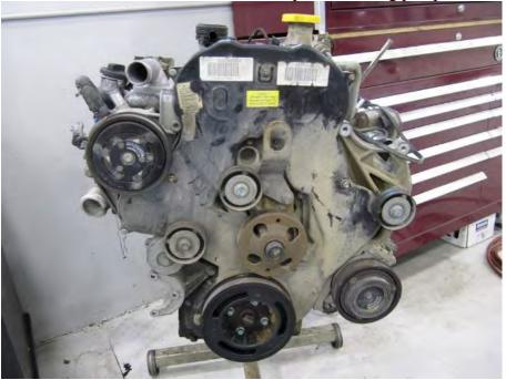
Glow plugs - Flow Control Valve intake elbow on left, IIRC #3 GP foreground and #2 barely visible in background. EGR valve is the thing with fins in lower center behind the pipe.
