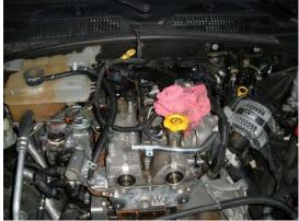
You have to remove 4 nuts to get it off 3 are easy. If someone has a tool that can reach the nut with the red arrow I will update this but for now here is how I did it...The top nut you can get with a socket. But the bottom nut I had to use a flex gear wrench and an adjustable wrench to get it off.
