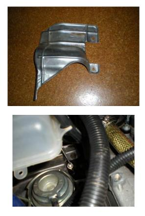
Run the sensor wires through the firewall, and I thought the obvious place was what I assume to be the clutch grommet (which is unused on my automatic).
