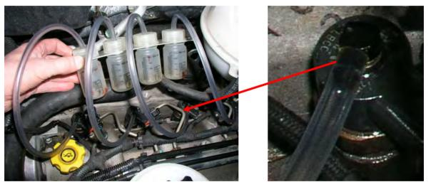
There should **not** normally be any fuel collected in receptacles during engine cranking.
