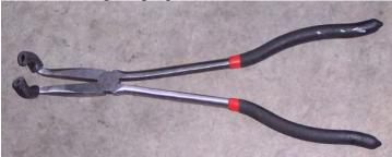
Long pliers are required to get at these. The picture shows hose pliers with vacuum hose for protection.
