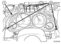
Fig. 3 Instrument Cluster Remove/Install
