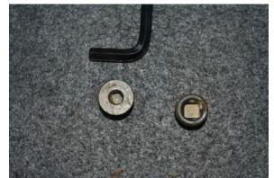
As you can see, the drain plug uses an allen wrench (10mm) but the filler uses some thing else that I didn't have soo....
