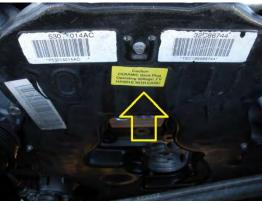
Find and remove the plugs in the valve cover. I had to use vice grips to break them loose the Allen wrench was striping out.
