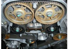
Make sure the fuel pump is aligned with the timing marks then using a pin wrench adjust the tensioner so the spring lines up with the notch. If you have a pin wrench from a VW TDI it will fit your jeep.
