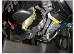
Ignition switch is white/black thing to right of steering wheel tilt release lever handle.
