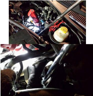
Once the top nut gets loosen up and moves to the top of the mount bolt, you will have to pull out the deep socket and replace it with the regular metric 18 socket, since (at least in my case) the deep socket is too tall and touches the FCV body.
