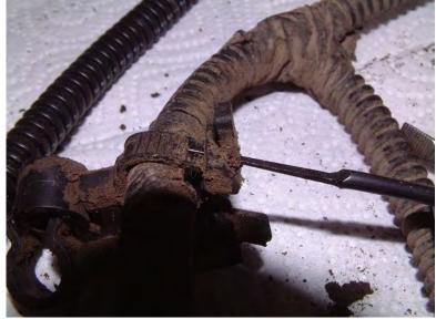
Here are the two ends of the harness rewired. I used 18 gauge wire; gray for hot and black for ground. As you can see, the 10-pin connector (right) is marked with pin #2 (the pump hot side). It goes to pin #4 on the 4-pin connector that connects to the tank. The black ground wire terminates in the passenger area and does not use the 10-pin connector.
