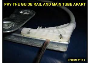
The side of the main tube that is facing up in Figure 11 should be facing down while you press the rivet through.)
