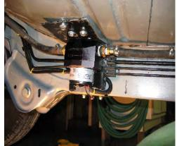
Here is the installed pump. I spliced into the 3/8" metal fuel line and used 3/8" fuel hose to connect the pump. I wanted to make the mounting bracket a little more protective but given the flow direction and mounting bolt configuration my choices were limited. The mount is rock-solid.
