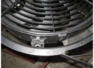
Here is the Haden 3814 mounted in the OEM fan shroud as viewed from the front of the vehicle. NOTE 1) the Hayden fan spins clockwise and 2) the finger guard seen here is on the engine side and cannot be removed as it's a functional part of the Hayden fan shroud. I used some hardware supplied by Hayden and mounted the fan by drilling through the bolt lugs and the OEM shroud.
