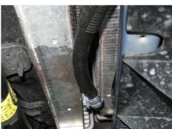
This is the line to the new cooler. I double-clamped it since the hard line isn't flared.
