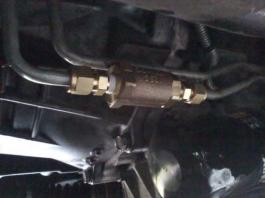
Here it is secured, I slit a piece of 3/8" vinyl tubing and put it on the top line, then tied the two lines together with a nylon tie, this prevents metal to metal from rubbing together, and stops vibration.
