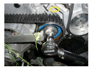
Then torque the cam sprockets...
