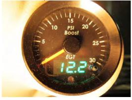
So far the highest egt I saw just fooling around a little was 715F. Normal driving is like 500F. Highest boost was 21psi with the GDE hot tune.
