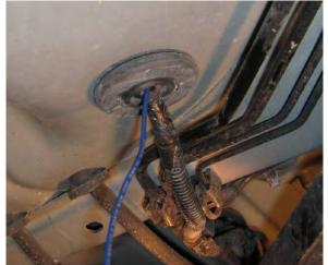
I spliced into the wire and ran the wire to the lift pump through the grommet under the left rear seat. It can be fairly easily accessed by reaching under the carpet and running your hand 'uphill' under the seat.
