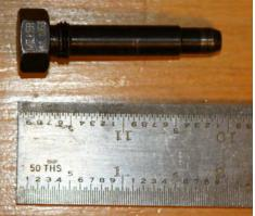
Miller 1053 - Exhaust pin - identical except as noted below Hex head - 0.58" across flats Overall length 1.932" Shaft length (base of hexagonal head to tip including threaded section) - 1.65" Shaft diameter of the thicker section is the same but the length of that section is only 1.25" of the above shaft length.
