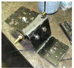
I mounted the pump using two bolts on the back and one on the top for three dimensional stability.
