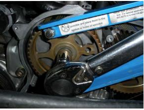
Do not use the locking pins to torque the bolts.
