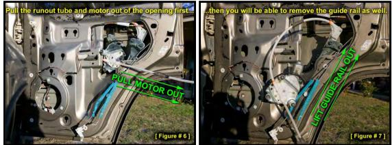
runout tube, the motor and the main tube through the opening such that the only part still inside the door is the metal guide rail. (*Figure 7*) At this point, you can lift the guide rail out as well. The next step is to disassemble the regulator.
