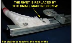
For clearance reasons, the head of the machine screw must be on the "metal" side of the guide rail, with the nut & lock washer on the "plastic" side, as seen here. [Figure # 13]
