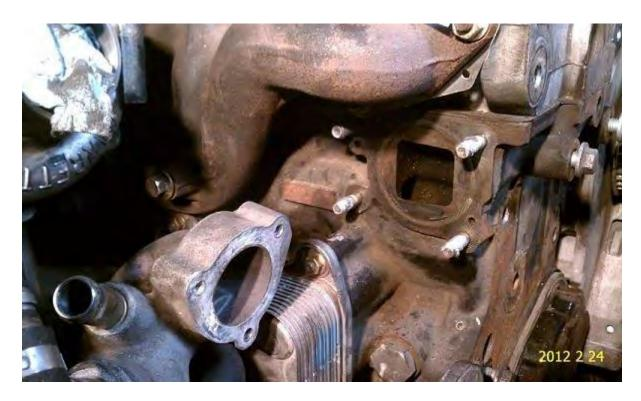
The three bolts on back, securing the manifold to the pump, are 8mm - and a 1/4 inch ratchet, universal joint, and 8mm 6-point socket worked well enough to pull them. Used a short extension to get a good angle on the top-rear bolt. Took a little juggling to get the right angles. I'd left the hose to the oil cooler connected on the bottom - if I'd pulled it the bottom bolt would've been easier to reach.
