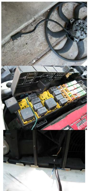
So far everything worked great. I then attempted to install the fan shroud and found that I had an interference with the hood latch hardware. I relieved this interference by cutting away a portion of the hardware and a portion of the Hayden fan shroud. The interference was overcome, but just barely (by ca. 1/8") and with more modifications than I am happy with. Here is the modified fan latch hardware and fan shroud.
