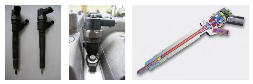
The fuel injectors are controlled by either a solenoid or piezo actuator.
