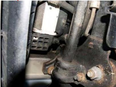
3. Remove the turbo to CAC/intercooler hose using an 8mm socket with extension.
