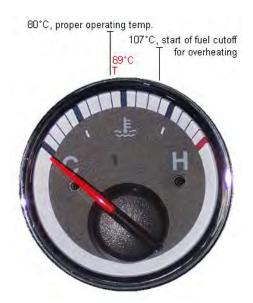
The thermostat should regulate the coolant temperature to 80C (176F). It is normal for temperatures to exceed this and go beyond center scale for hot weather driving, hills and towing. Note that the indicated 89C (192F) mark is for the modified thermostat if you have one.
