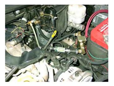
This is a picture of the lift pump installed. Note the inline fuel filter before the pump.
