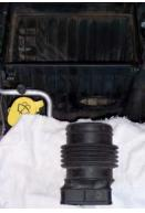
Remove the intake duct from the airbox. You may need to spin it 90°.
