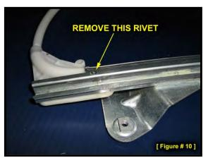
At the top of the guide rail (where the main tube attaches) you will find a small rivet. (*Figure 10*) Remove the head of this rivet. You can use a drill, grinder, cutoff wheel, Dremel® tool or even a hand file if you have the elbow grease to spare, but whatever method you use, be careful to only remove the head of the rivet itself; do not damage the underlying metal guide rail.
