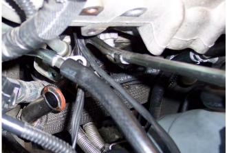
For re-install, the EGR pipe should have high temperature RTV Silicone re-applied (Permatex Red, or Orange as a 2nd choice).
