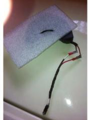
OEM amp with ethafoam pad mounted and wireing pigtail installed.
