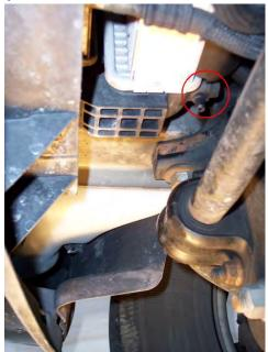
The engine should be cold for this procedure. Turn the cabin heat on to full (engine not running). Disconnect the battery. Attach a 5/16 inch hose to the radiator drain cock. It is on the inside, passenger side, lower corner. Feed the hose into a clean bucket; we will save the coolant.
