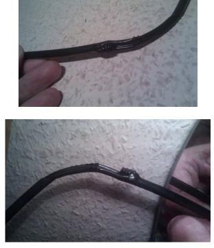
here are some aditional pics of the Line. it is the one with slighly larger diameter, which is connected to the solenoid by downward U flexible tube. the point were it is melted is indicated by the knife:on that pic the 2 lines from the solenoid are still taped together, the protectors are removed. the one damaged is the larger and shorter line with the downward U at one end
