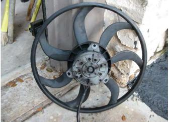
The Hayden 3814 fan. Notice the three fan lugs (white dots) on the Hayden match the OEM fan lugs but cannot be used because the fan would spin the wrong way.
