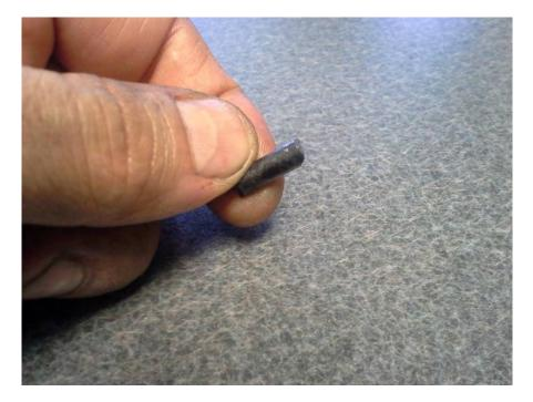
I didn't use the ID parts adapter (won't fit per "cevans" at ID parts); I put mine in the intake manifold. It's a preexisting spot that you need to drill a small hole into (I asked but he did not recall size of drill bit - blow or vacuum shavings as they come out and carefully pull bit out to avoid shavings in intake). I'm not sure what size threads it is but I had an adapter from a Dodge Cummins that fit.
