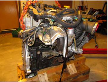
Passenger side view showing rear unused oil port (this can be used to mount an oil pressure sensor in the upper engine pressurized oil gallery "before" the turbo oil feed), turbo supply line and on the left rear the crank position sensor with heat shield removed for access
