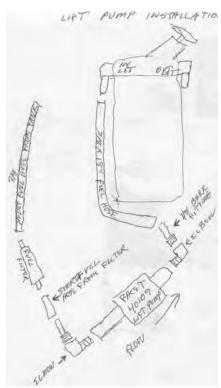
This drawing is the illustration of the lift pump install
