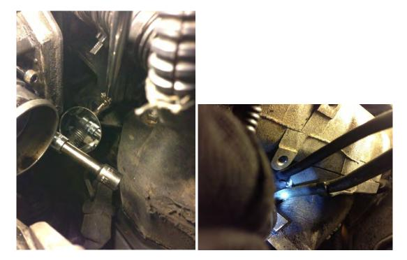
Try sticking the hand in between the elbow and cylinder head, you can use that hand to drive the socket to the bolt while the other hand to untie the bolt with the socket and flex head drive.
