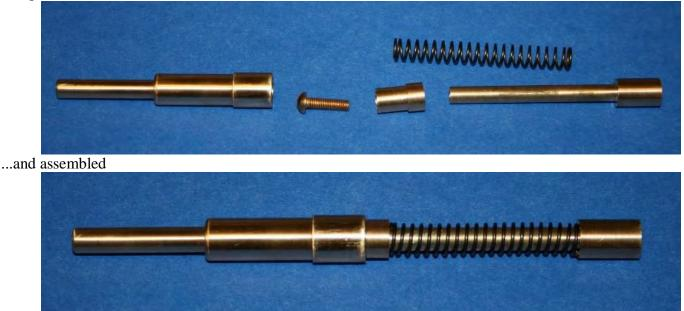
Of course, you could replace with a solid rod. Maybe a chopstick cut to the correct length and do away with the spring altogether. The spring simply allows the rod to "give" if you push the release button on the shifter lever
