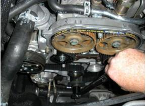
Recheck the tensioner it will pull the slack out of the belt and will most likely have to be readjusted.
