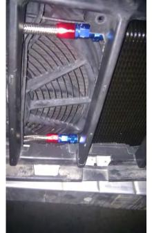
See how the plastic is trimmed to allow the cooler to pass behind
