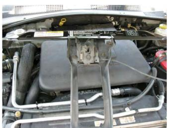
The notch is cut into the front of the fan assembly and the reinstalled removable finger guard.
