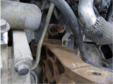
Cam notches aligned - engine in time
