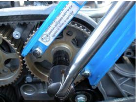
Now remove the bolt on the tensioner and the tensioner then the timing belt and the cam sprockets and the two idler pulleys TURN THEM CLOCKWISE TO REMOVE THEM. **NOTE: the next picture shows the cam ends with the sprockets removed.** Notice the 2 notches in those cam ends that face each other with the engine in time, same notches in same postion show in a picture from Eugene Buford who confirms that his picture was taken with the 2 cam pins and the flywheel pin installed.
