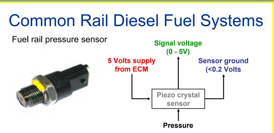
Typical signal voltages from rail pressure sensor:
