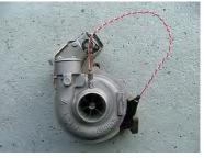
> Front View of the turbo assembly, with optional speed sensor installed.
