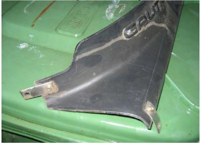
Top view of cut edge of shroud from front of vehicle
