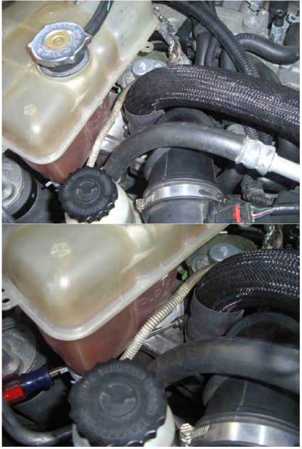
3. Remove the clean air duct by loosening the screw clamp at the air box and at the inlet to the turbo compressor. Also remove the hose that goes to the CCV outlet on the engine. Remove clean air assembly and set aside.
