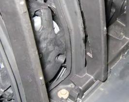
I notched one of the posts to allow the cooler to fit flush against it.
