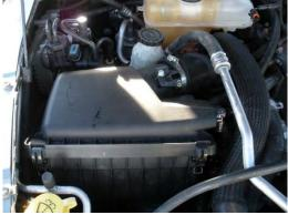
If the grommet comes out put it back into the finder it makes it easier to put the air box back later.
