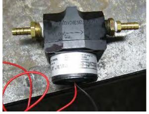
I ordered the Kennedy lift pump from <u>Kennedy Diesel</u> (the fittings weren't included). It is a centrifugal type which won't cause a restriction if it fails.
