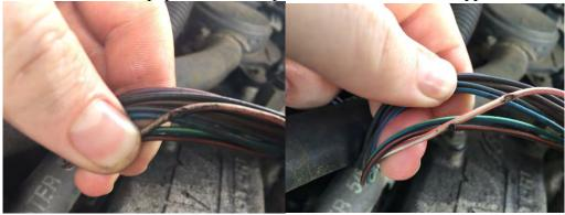
Wrapped some 3M super 35 tape around the wire and then put on new loom protected by more yellow super 35!
