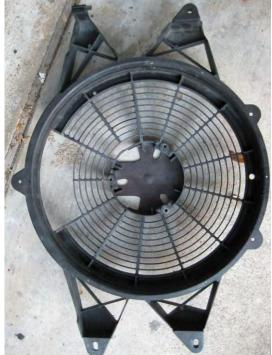
The fan (front of vehicle side). Notice the three lugs for mounting the fan
