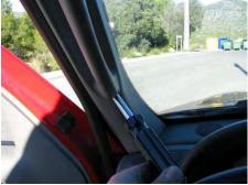
(2) Remove the instrument panel top cover. (lift the left side only to access cluster screw)
