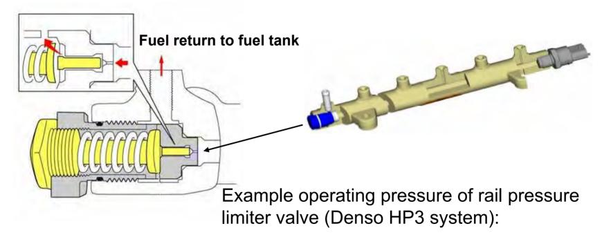
valve opens at 230 MPa (2300 Bar) valve closes at 50 MPa (500 Bar)
