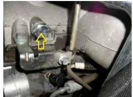
VM.1053 is just behind the thermostat housing about in the middle of the valve cover. After getting the cam locking pins in with the fuel pump either lined up or marked you will need to jack (**NOTE - no need to do this for just timing belt job**) the jeep up enough to get under it USING JACK STANDS not just the jack.
