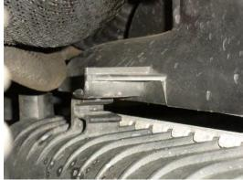
Remove the fan and shroud carefully don't drag the fan against the radiator.
