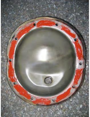
So here came the problem. The gasket kept moving around when I was trying to bolt the cover back on so I decided to use some old RTV i had laying around to hold it in place.
