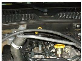
Remove the two bolts holding the shroud lift it up. (NOTE - the nuts for these bolts just slide in/out of retainer clips on the radiator so are easy to lose. May want to glue or zip tie into place)
