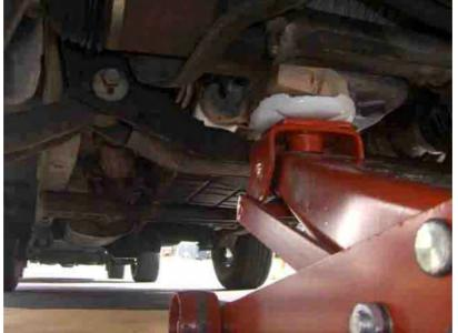
8. Now the engine mount can be pushed up enough from underneath the vehicle to free it from the engine mount bracket. The mount can slide down next to the exhaust pipe and engine block to be removed. You may need to push the transmission cooler lines outboard a bit.
