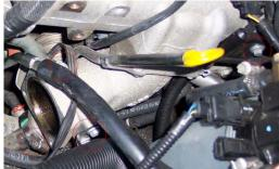
Loosen the clamp (7mm) on the EGR pipe enough to slide it off of the flange and down the pipe. Remove the pair of 10mm bolts shown holding an electrical cable bracket. Remove the (long) 8mm bolt at the far right.
