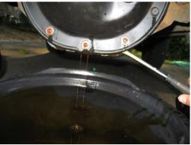
I untightened the screws and used a flat head screw driver to pry open the pan.
