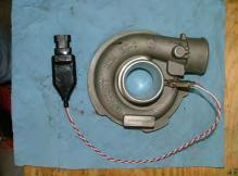
Up-close of modified turbine housing. This shows where a new flange corresponding to the KJ manifold (cut on waterjet machine) has been tig-welded onto the housing to properly orient the turbocharger once installed on the engine. This picture does not show it, but the throat of the housing (just after the flange) will be drilled and tapped for a thermocouple probe installation (all units will be
