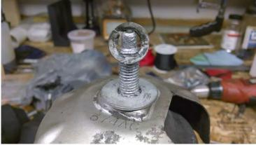
This picture has the heat shield on the new mount, and I ended up using a 1/2 washer to replace the "factory" one that somehow was cracked (and not by me for sure). You can see the factory washer on the top of the upper bolt. The new 1/2 washer would definitely resist better than original.
