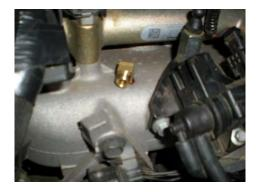
Boost line installed to sensor:
