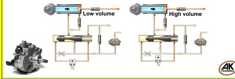
Fuel metering control valve failure symptoms and diagnosis
