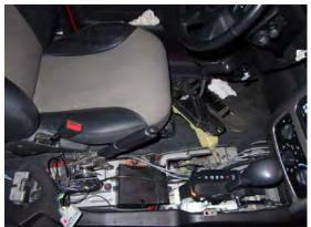
Now after you remove the 4 10mm nuts from the TC shifter you can pull it up and out as you try to move it out of your way the best you can. Then look down in the hole and you see the sensor.
