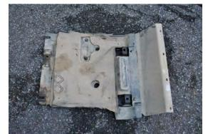
took off the engine skid leaving the radiator skid attached. Notice the plastic cover on it? I'm very surprised i didnt find any beach sand or rocks under it when it took the plastic cover off. OH WELL its not going back on!
