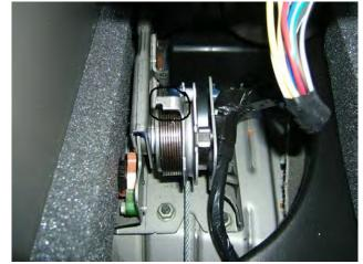
When you pull the ebrake up, that entire thing will move with it. When you hold the tab and let the handle back down, it will stay in place. Max time: 15min
