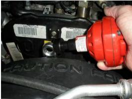
When you get it off just leave it in the shroud they have to come out together. (NOTE - probably a good idea to put a towel between fan and radiator to prevent nicking radiator core and causing a leak)
