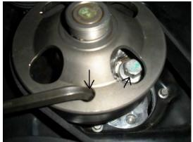
Cut the zip ties off the Freon line and overflow line.
