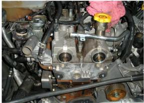
Install the back cover and the cam sprockets leave them loose then the idler pulleys and the tensioner then the timing belt. Not all torque wrenches work backwards keep this in mind when you put on the idler pulleys.
