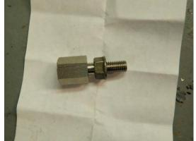
I drilled the manifold with a 5/64 bit, put some pipe dope on the threads and installed the boost bolt. I snugged the nut downward to keep it tight. The Mcnally MAP sensor is installed with some pipe tape. I used wire conduit for everything for a factory look. You can hardly pick out the new sensors in the engine bay.
