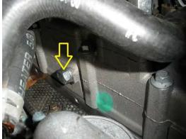
Now install VM.1089 into the flywheel located under the jeep you don't have to take off the skid plate it's kind of hard to see so a good light will help it goes in the housing at the back of the engine where the transmission bolts on you can see the tail pipe to the left of the picture.
