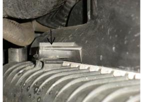
The bottom is held in place by this slot and groove it just pulls out...
