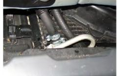
The new cooler outlet is connected to the factory line. I used plenty of ziploom to protect the lines.
