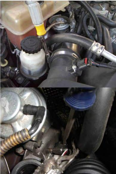
4. Now you have access to the top engine mount retention nut. Remove this using an 18mm socket, with a universal joint and 24" of extension.
