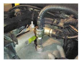
Here you can barely see the hole I cut in the turbo heat shield to pass the thermocouple wire through. It goes in to a 1/8 NPT compression fitting where I drilled and tapped the manifold in the same way as warp2diesel. (Thanks for posting that diagram). I didn't run the engine while drilling or anything like that. just a shop vac right near the hole and a small magnet down in afterwards.
