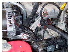
To gain access to #2 glow plug, remove the alternator rear "T" bracket (13mm and 15mm). Squeeze the black tab (red arrow) and unplug the harness connector to the glow plugs. Flip the bracket out of the way.
