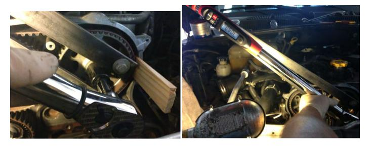
Remove the pins from fly wheel and cams, test your timing for few complete turns and you're good to go.
