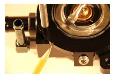
**Thermostat valves that fit the model 001:** Any thermostat valve that fits the 5.7l, 6.1l, 6.2l, and 6.4l hemi Chrysler V-8 engines will fit in the Model 001 assembly. The following are 2 lists of thermostat valves that will properly fit into the hot diesel solutions model 001 engine thermostat housing. These lists feature companies that manufacture the hemi v-8 engine thermostat, or are re-branded thermostat valves from other manufacturers.
