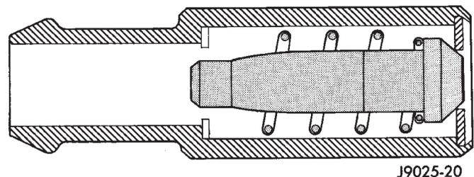
Fig. 6 Engine Off or Engine Pop-Back—No Vapor Flow
