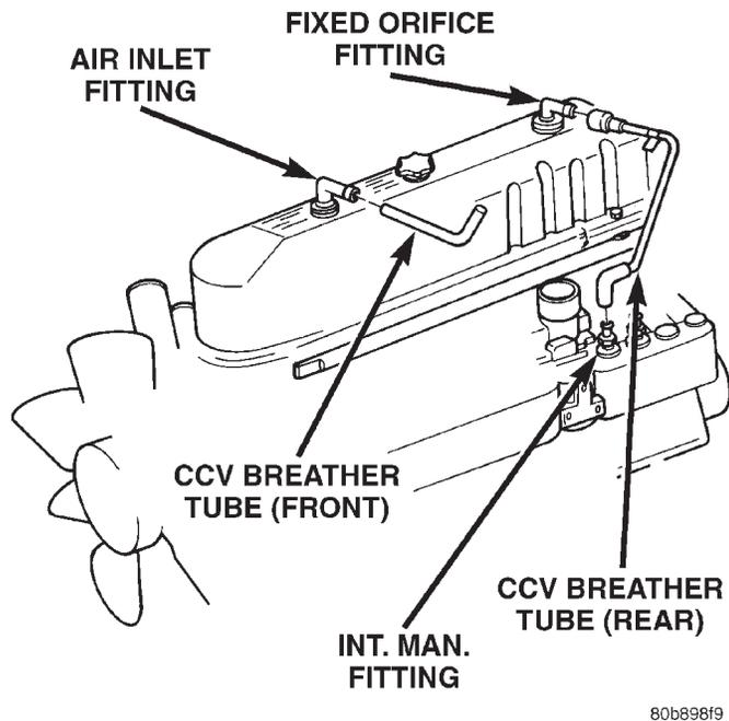
**Fig. 10 Fixed Orifice Fitting and CCV System—
