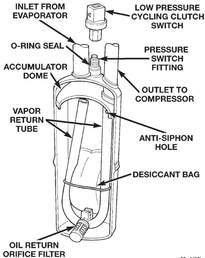
**Fig. 1 Accumulator - Typical**
