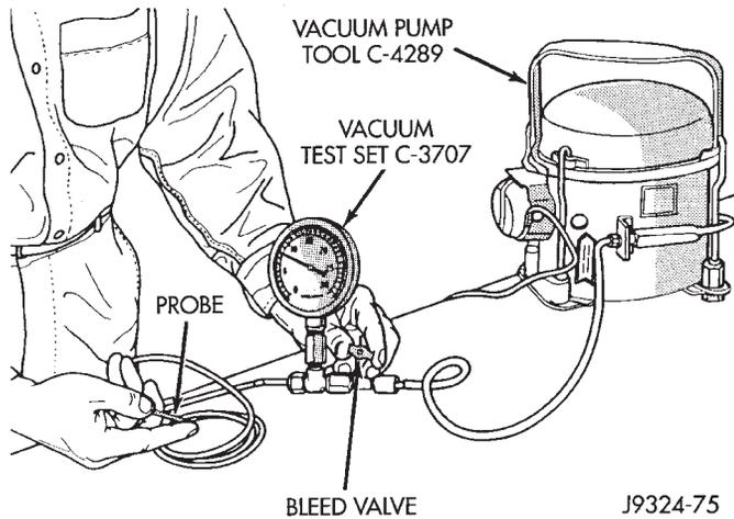
**Fig. 7 Adjust Vacuum Test Bleed Valve-Typical**
