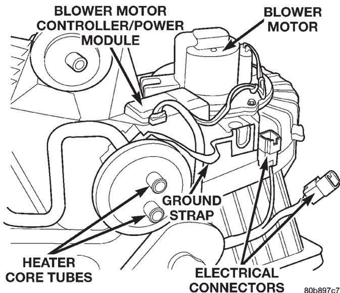
**Fig. 27 Blower Motor Resistor or Controller/Power Module Remove/Install**
