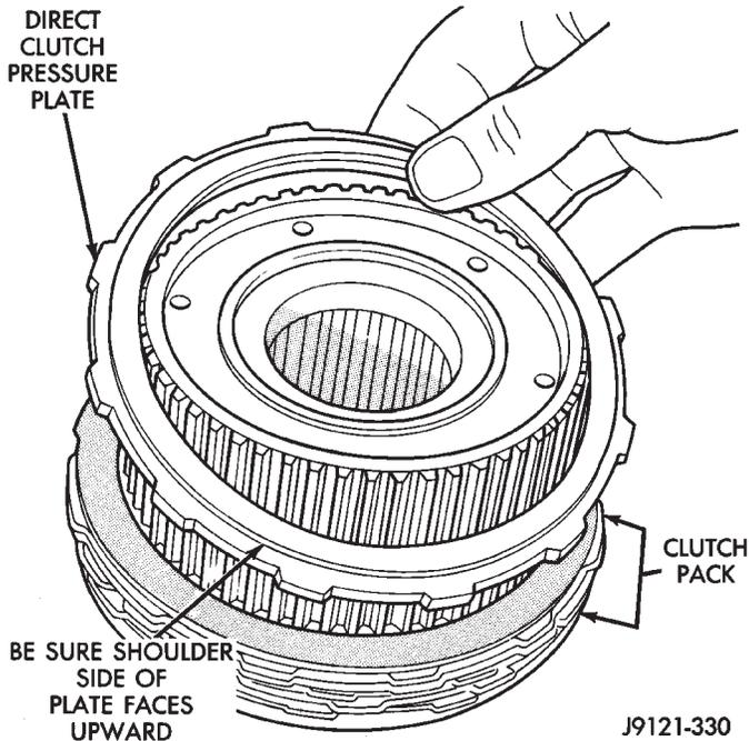
Fig. 249 Correct Position Of Direct Clutch Pressure Plate
