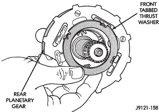
**Fig. 194 Installing Rear Planetary Front Thrust Washer**
