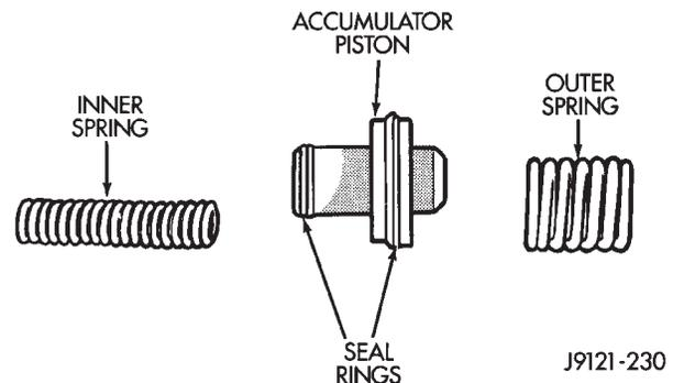
Fig. 266 Accumulator Components
