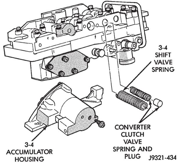
**Fig. 81 Accumulator Housing, Valve Springs And Plug**
