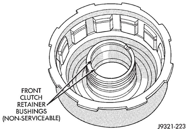
**Fig. 269 Retainer Bushing Location/Inspection**
