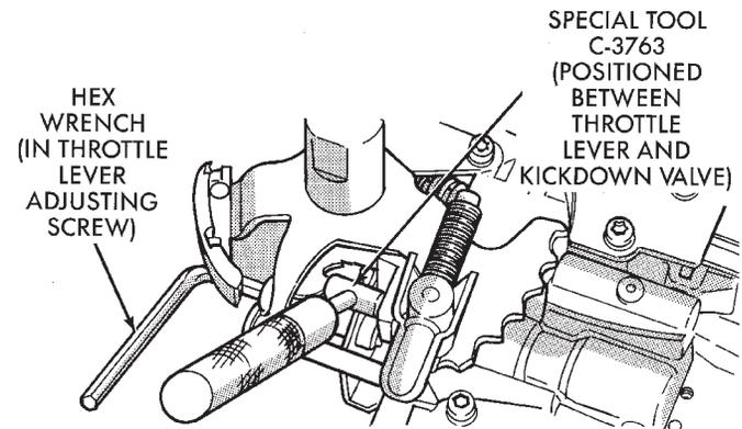
**Fig. 281 Throttle Pressure Adjustment**
