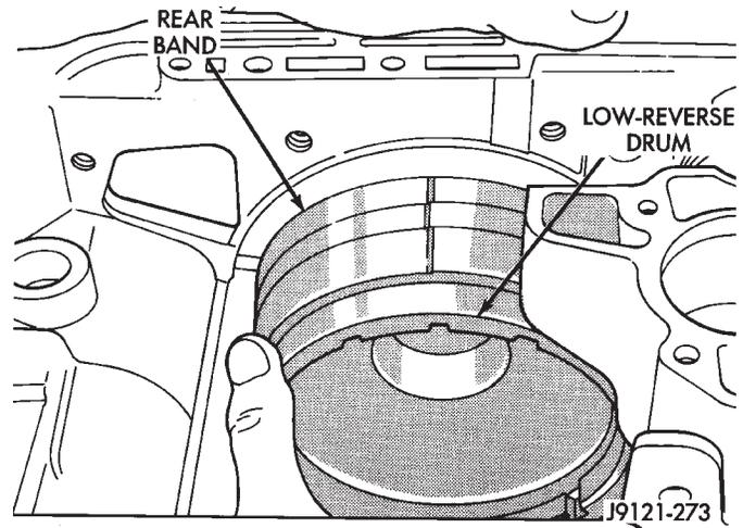
**Fig. 135 Installing Low-Reverse Drum**
