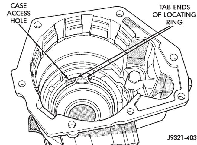
**Fig. 255 Correct Rear Bearing Locating Ring Position**
