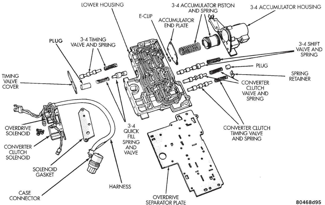
Fig. 93 Lower Housing Shift Valves And Springs
