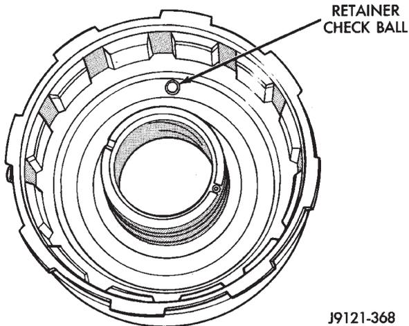
**Fig. 268 Front Clutch Piston Retainer Check Ball Location**
