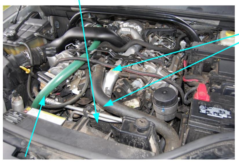
Remove bolt and screw so you can loosen this silver pipe. See next slide for details.
