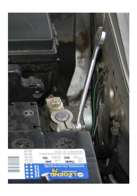
Remove the negative pole of the battery as always.
