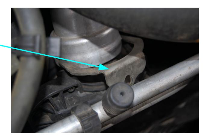
There are two more 8mm bolts and one more clip that holds the turbo resonator on. To remove the top bolt, use your small ratchet with extensions and universal. After you get it loose you can pull it out with the flexible grabber. This is the most difficult bolt. It is hiding down there right under the belt.
