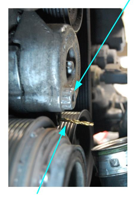
Using the 1/2" breaker and 17mm socket, turn the belt tension device a small amount and place a nail, or drill bit into the locking hole. This will hold the tensioner while you work on the belt. Do NOT remove the tension device or the pully that is attached to it. You are turning it counter clockwise, moving your wrench from the passenger side toward the driver side. You are only rotating it about 3/8 of an inch but it is a pretty stiff pull.
