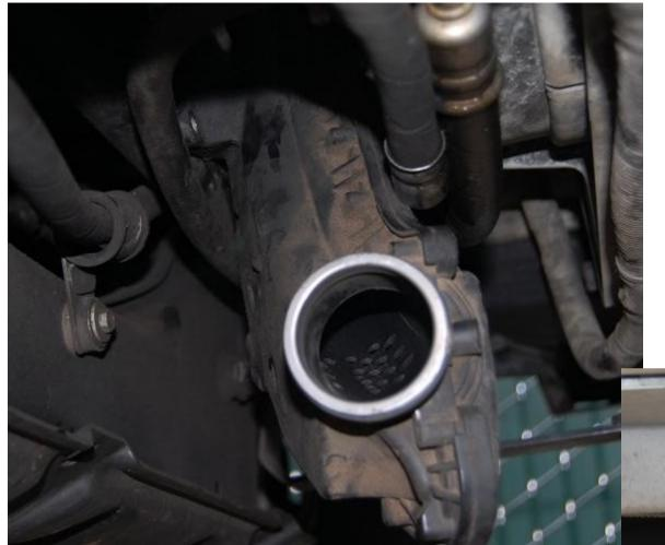
After you remove the clip, pull the intercooler pipe off of the resonator.
