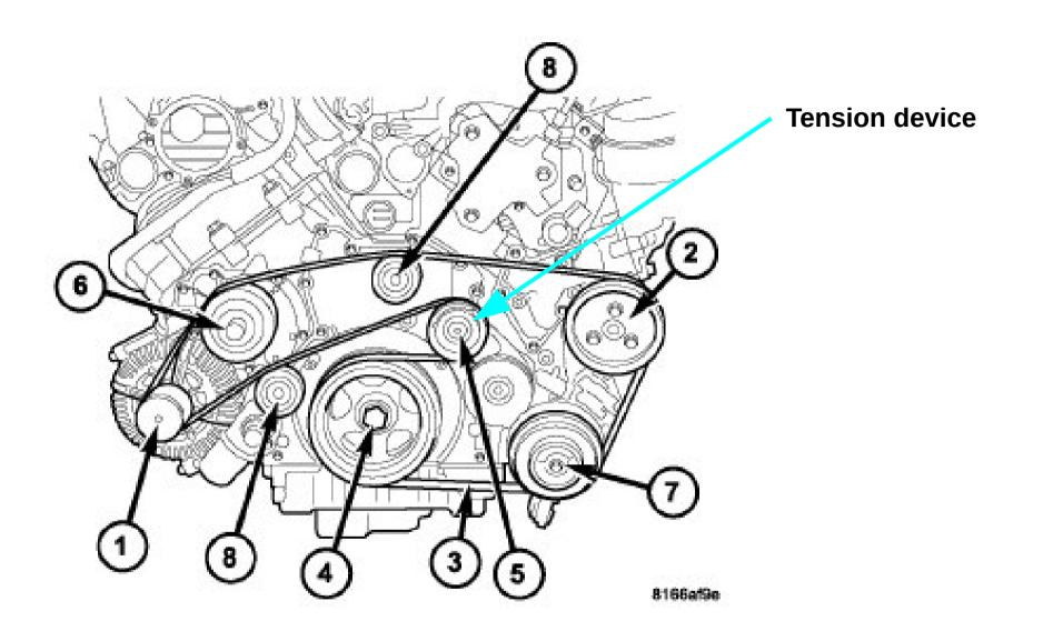
Compare your belt to the diagram until you fully understand how it goes. Remove the belt. Inspect all pulleys for wear.
