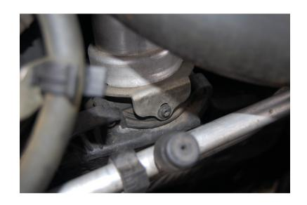
After you remove the screw, slide the flat C shaped clip off. Slide it straight forward toward the front of the Jeep. You can now lift the silver pipe up a small amount disengaging it from the turbo resonator although it is better to wait until the resonator is loose too.
