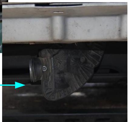
This is the resonator. I thought about gutting it out, but changed my mind. Put the snap ring back on the resonator now. When you replace the intercooler hose, it will just snap into place. If your resonator is all gunky, clean it. Mine wasn't.
