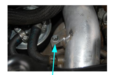
Loosen but do not remove the pipe that connects the turbo to the turbo resonator. If you remove this pipe, you risk ruining the O-Ring seal that connects it to the turbo.
