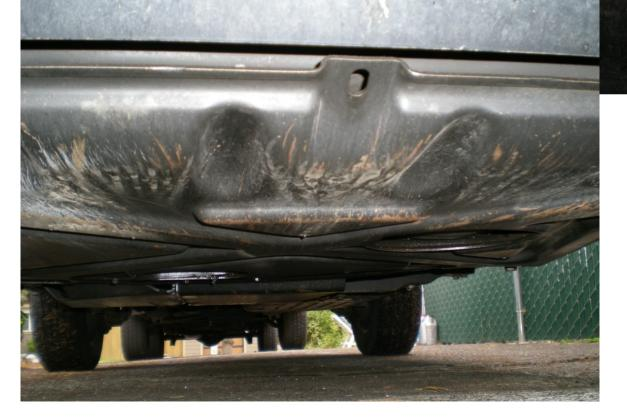
Remove engine skid plate if you have one. Mine is a factory skid held on with 4 bolts. Loose the two in the front. Remove the two in the back.
