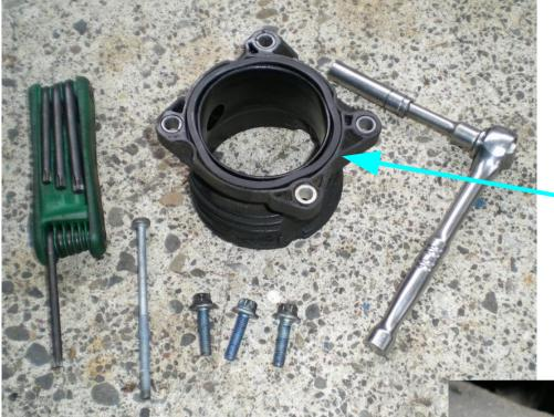
You do not have to remove the entire throttle body, just this plastic extension tube. Replace the gasket with the new one if you purchased it.
