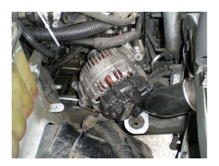
Now for the big fight. Move the alternator forward to clear the throttle body and nose it down while rotating it to clear the AC line. Gently pull the AC line a little and keep wiggling around until you can back the alternator out of the hole. Keep working it. It IS possible. I did this by my self without a helper. Its heavy and it is a very tight fit but keep at it and you will get it.
