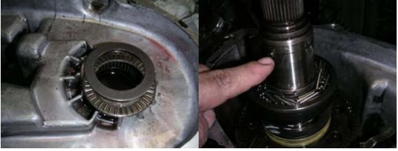
Note the bearings and this thin shim must go back in same place. note hi-range shift ring
