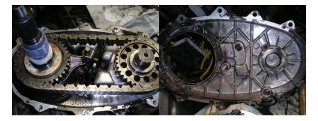
Make sure you note all the shims and the Torrington locations. You can see one bearing in the lower left pix on the right sprocket and a shim on the left shaft. This has a good chain.
