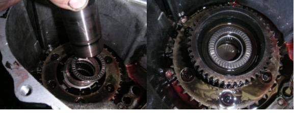
The last pix are showing the detent (Left) and lock bolt (right) that hold the shifter plate in position. You will need to grind the bolt shorter so the plate can move or add the stock ball switch if you want a "4x4 engaged" Light.
