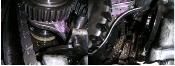
Lift off the chain and gears as a unit, all the bearings will fall all over, DO NOT LOSE ANY!!!Note the Torrington bearings and all the roller bearings that fell. Also notice how shiny all the bearing surfaces are, no pitting, blue marks, or metal transfer, it all looks mirror smooth. This case is in excellent shape and shows no abuse from 23000 miles in low range. I think it will go 100,000+ as it is and running in low doesn't hurt anything like some say since the planetary
