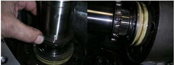
Next pull out the shaft and note more bearings they are all shinny and mirror like as is the shaft. None need replaced but I will replace all the seals. You can now see the gear that locks the outer part of planet gear so you can get hi range. You will also have to cut the snap ring off the shaft just above the plastic shift ring. It is the smaller on the main shaft
