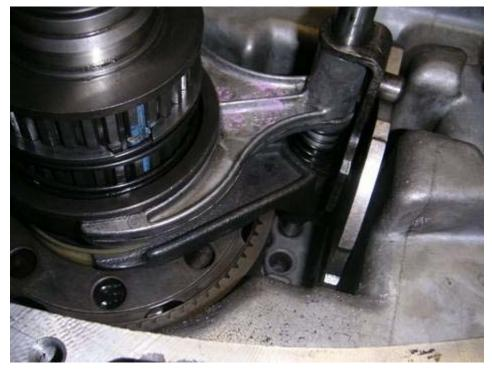
Again add the gears and with 2 guys and a monkey put the chain on, and add the torringtons to the case with the thick shim towards case then bearing, and then the thin shim. Don't forget lots of white grease...
