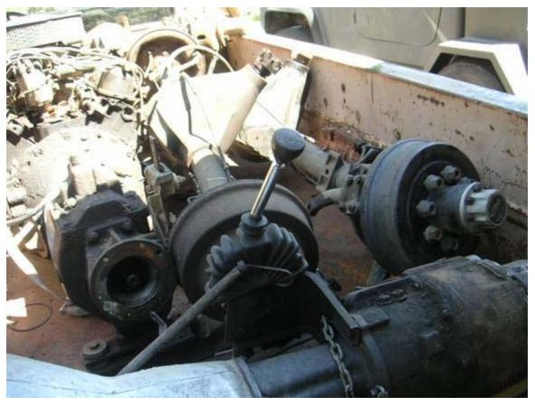
Almost have enough parts! Notice my Dana 70 front and rear axles. This will get a 440 stage 6 with an auto bolted to a NP205 and Dana 70 front and rear with lockers and 4:88 gears so stay tuned!!!
