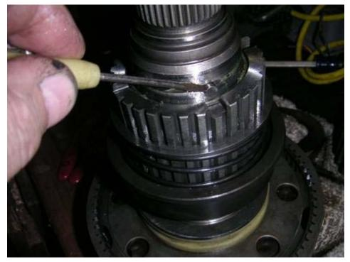
Put the chain gear on the spline color before the snap ring goes on. I did it wrong the first time and forgot the sprocket...and drop it all in the case with the forks engaging the plate like this. Don't forget the Torrington bearings in the case!
