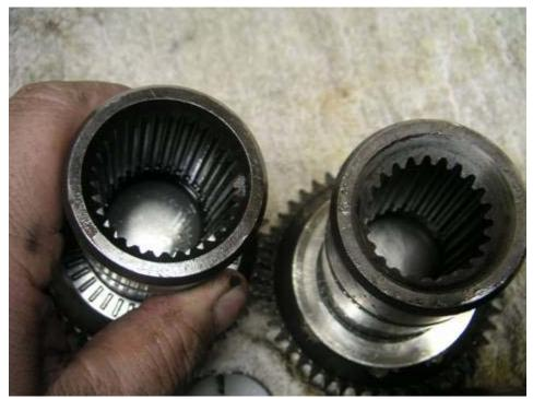
You cant use the ford shell as it is too long and hits the low range gear in bottom of case so You cant just swap out the hole plant assembly as some have suggested they did...
