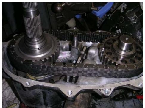
Colored link goes out and don't forget the magnet! Add the other case half bearings and bolt together with sealing goop. Then add oil pump and Speedo collars with the white oil pump groove down and push till it gets flush like this.
