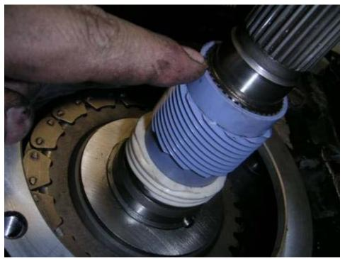
Add oil pump plate with white grease holding it in the slots and bolt on. Hopefully your output yolk looks like this with NO groove you can feel with your finger nail. If it has a groove don't pound the seal in so far and it will have a new place to ride on or get a speedy sleeve to fit the shaft.
