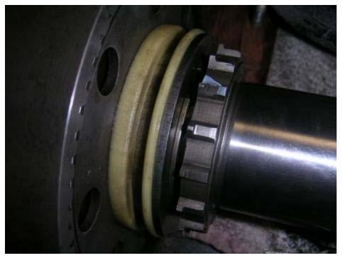
Here are the parts you scrounged up. First notice the new plate on right has the slot for the hi range fork tug plate is left and has no slot. Notice the plastic rub tabs on the ford fork. You need a fork without this feature or weld them up and file slots smooth so they don't eat the nylon shift collar.
