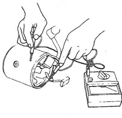
Figure 5-17. Coil-to-Frame Continuity Test
