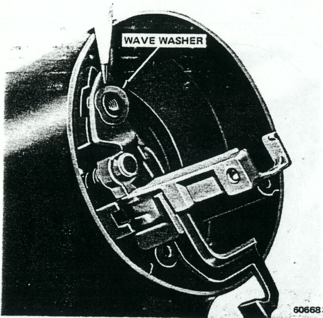
Fig. 2J-13 Wave Washer Position
