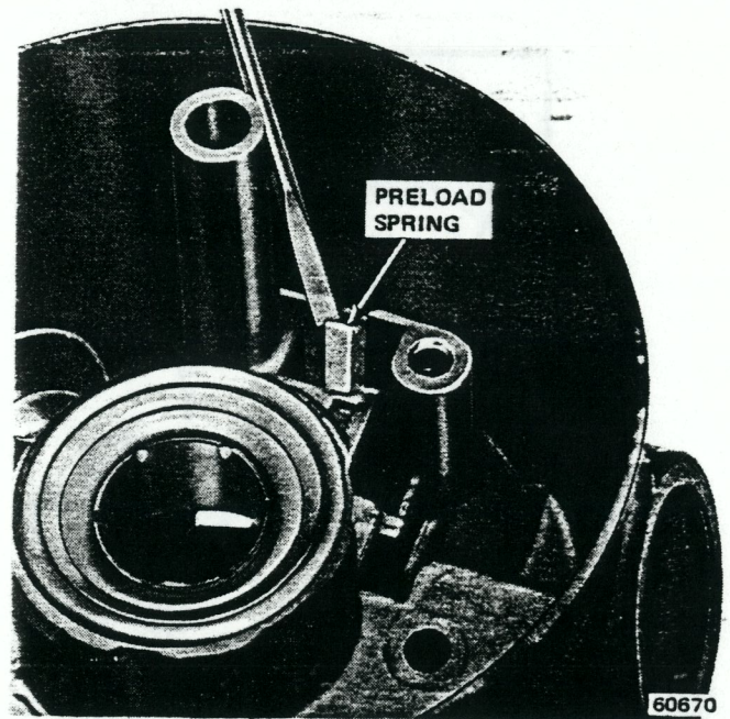
Fig. 2J-15 Rack Preload Spring Removal/Installation
