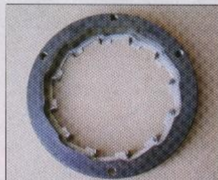
A-1 offers a bolt-in overrunning clutch for 727 TorqueFlites that offers better support for this inherently weak area. The piece begins life as a stock unit, which is then drilled and tapped. Even when beefed up, it's never a good idea to do a burnout in First gear with a TorqueFlite transmission.
