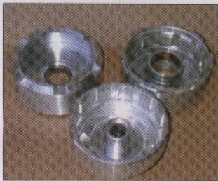
A-1's ProFlite transmissions feature ultralight-weight innards like these aluminum drums, but that doesn't mean they're weak. These transmissions live behind 1,300hp NHRA Comp Eliminator cars.
