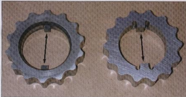
Another breakage-prone area of the 727 are the drive tangs (arrows) on the inner pump rotor. The tangs can break off if an engine kicks back after shutoff. High-compression race engines are more prone to cause this than low-compression street pieces. A-1 makes inner pump rotors with larger, heavier-duty tangs.
