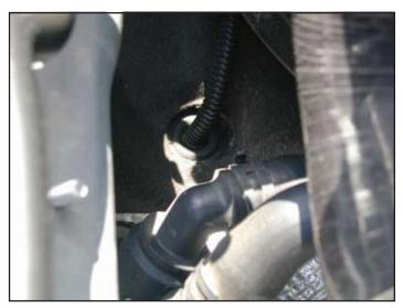
Another unused grommet is located to the upper left of the brake booster. In this image a piece of black wire loom has been pulled through the grommet already.
