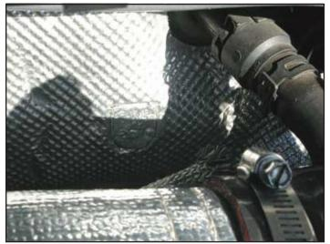
An unused grommet can be found through this opening in the heat shield at the back of the motor. You will need to pull this precut opening in the heat shield to access the grommet.
