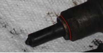
Use a vise to hold the flat part of the injector body - put a paper towel around the base in case fuel leaks out. (It also keeps the injector clean since my vise was dirty). If you are thinking of just holding it with pliers you are asking for a dropped/dirty/damaged nozzle. All four of my injectors also needed a breaker bar to loosen them, so some sort of vise is a must here!
