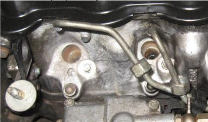
The sealing washer will be stuck on to the injector with soot. I suggest using pliers and turning the washer a 1/4 turn with a light pressure. This will break the carbon buildup and the seal. Don't go near the retaining nut's sealing surface to avoid scratching it (marked with a red line below). Don't use a screwdriver or pick to remove the washer because this can scratch the surface! Clean the exterior of the injector as much as possible.
