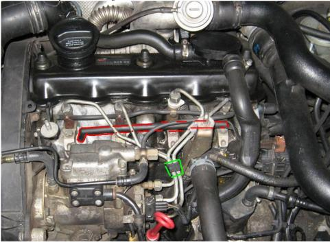
Use a screwdriver to remove the black plastic clips (outlined in green above) holding the pairs of metal fuel lines together. Some cars have a metal clip.
