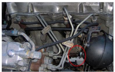
Remove the 4 injector holders (the metal fork holding the injector) and place to the side. There is 1 conical washer on each injector holder and they are each held by 1 x 13mm bolt (circled in red below). In the below picture I removed a glow plug to do a compression test and hadn't yet cleaned the other spots or removed the fuel
