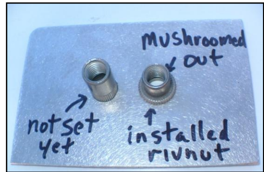
Figure 40 - The rivnut will mushroom out and expand
