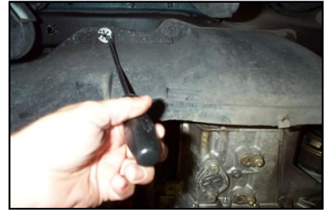
Figure 55 - Tighten the star nuts further by placing a flat bladed screwdriver in one of the star nut's radial slots
