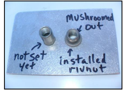
Figure 29 - Rivnuts are locked into the body by setting them
