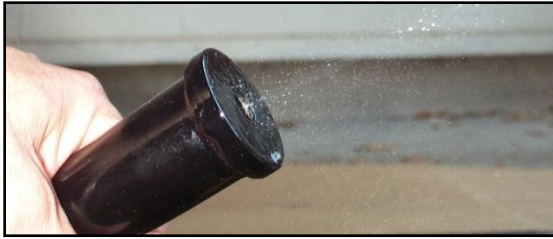
Figure 48 - Spray the female threaded hole of both of the front mounting posts with WD-40 or equivalent spray
