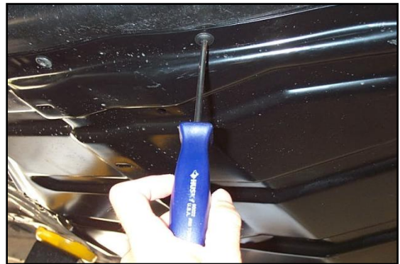
Figure 21 - Removing all of the Torx T25 screws
