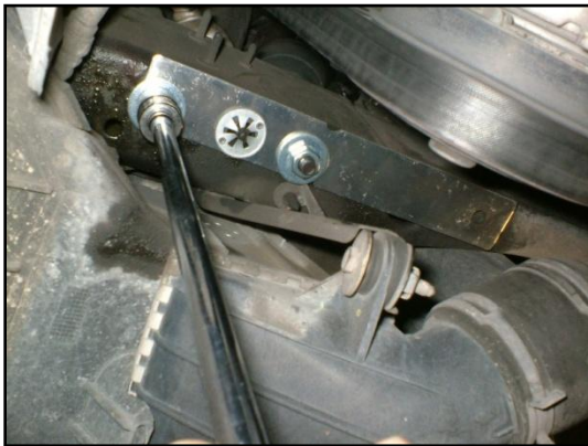
Figure 46 - The star washer will help keep the rivnuts firmly against the frame rail when you tighten the nuts
