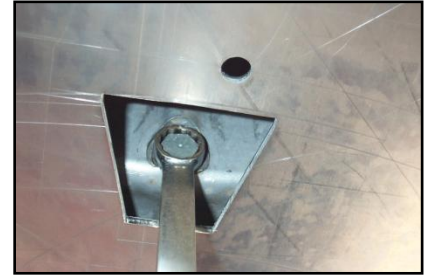
Figure 62 - Use a 19mm or three quarter inch wrench or socket on the drain plug to loosen the plug
