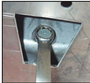
Figure 56 - Trapezoidal keystone shaped cutout for draining your oil through the bottom of the car.
