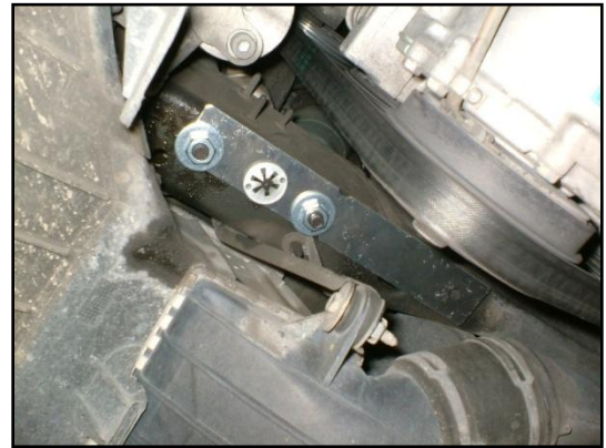
Figure 45 - The "tail" of the rivnut tool will go toward the rear of the car .
