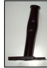
Figure 49 - The post is not welded perpendicular to the base plate
