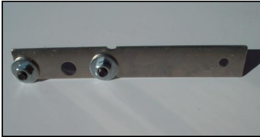
Figure 44 - Insert the studs through the rivnut tool on the side opposite of the stamped letters
