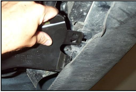
Figure 53 - Sliding the front rounded edge into the slot in the radiator support
