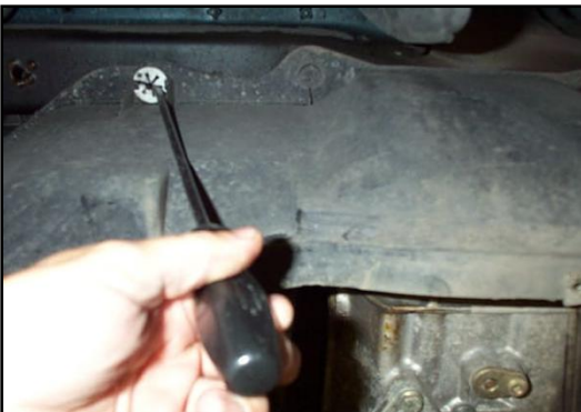
Figure 22 - Unthreading the flat star speed nuts with a long screwdriver
