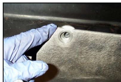
Figure 63 - Slip the last extra washer between the skid plate and the rear center bolt hole
