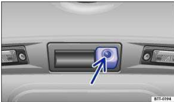
Fig. 264 In the rear hatch: Location of the Rear Assist camera.
