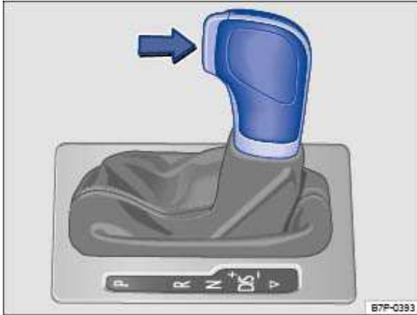
Fig. 244 Automatic transmission selector lever with shift lever release button (arrow).
