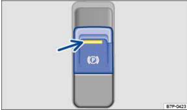
Fig. 246 In the lower front center console: Button for the electronic parking brake.
