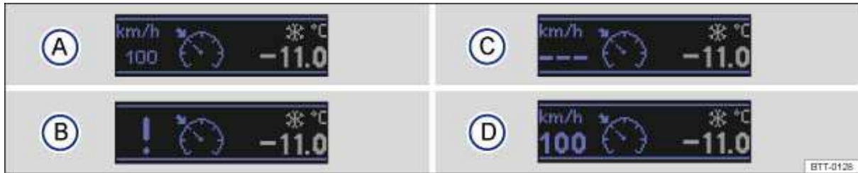
Fig. 133 In the instrument cluster display: Cruise control status indications.
