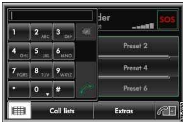
Fig. 225 Entering a telephone number.
