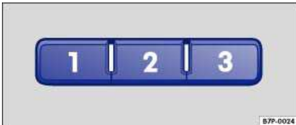
Fig. 37 Roof keypad: Buttons for the HomeLink® Universal Transmitter.
