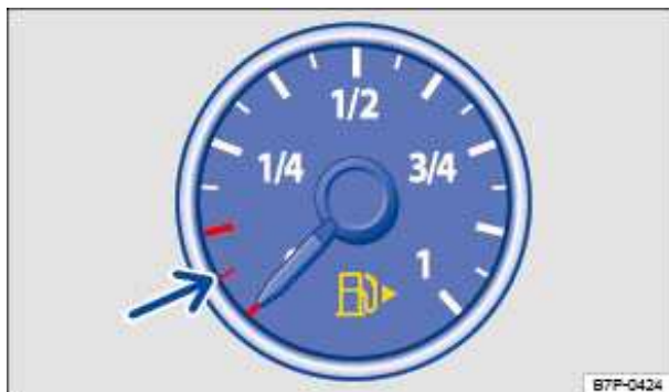
Fig. 275 In the instrument cluster: Fuel gauge for gasoline and diesel fuel.
