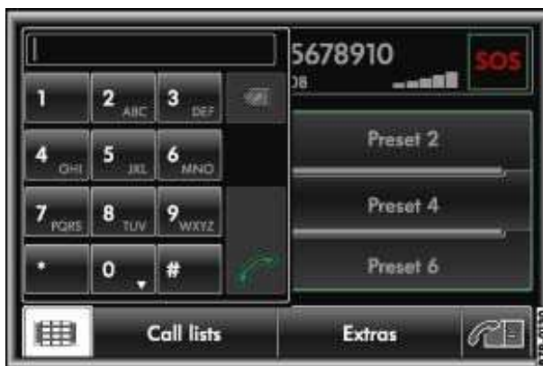
Fig. 235 Entering a DTMF button tone during a call.
