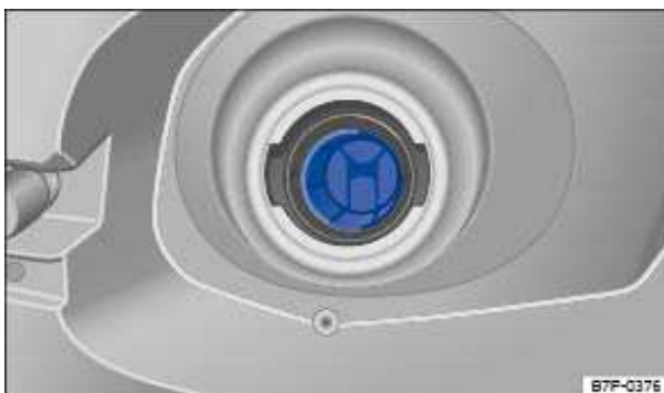
Fig. 278 With open fuel cap: Misfueling guard in the fuel filler neck
