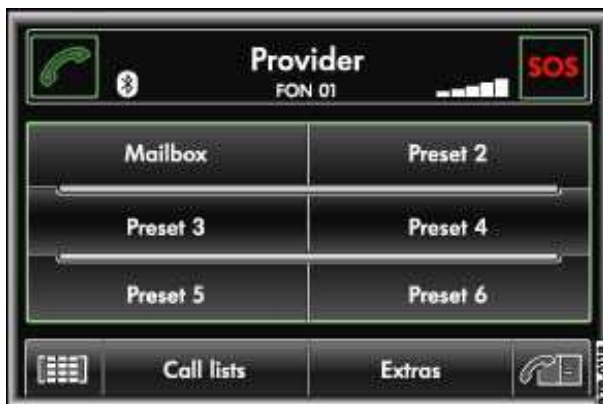
Fig. 223 Telephone control main menu.
