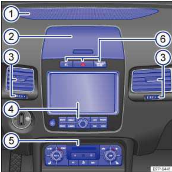
Fig. 6 Overview of upper front center console.
