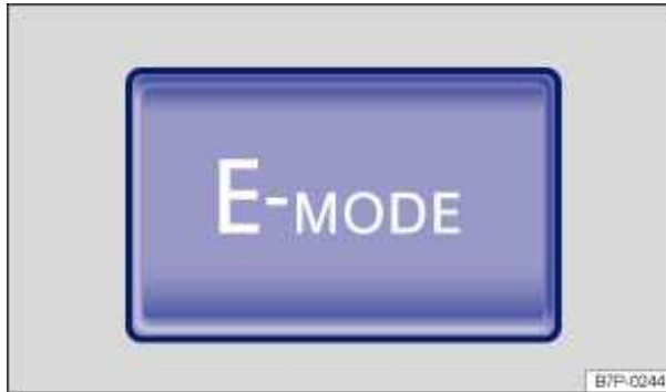
Fig. 251 In the lower front center console: E-MODE button for extended electro-mode drive.
