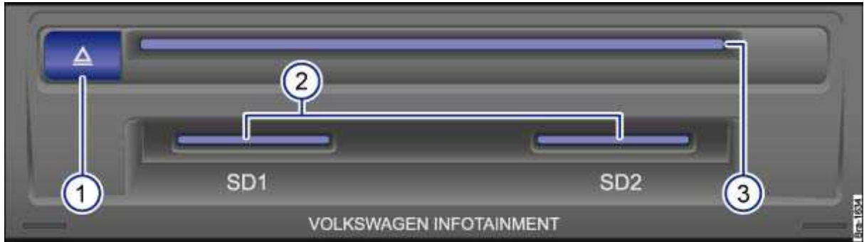
Fig. 143 Data media slots in glove compartment.
