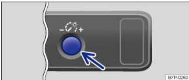
Fig. 85 Next to the steering wheel: Control for instrument cluster lighting.
