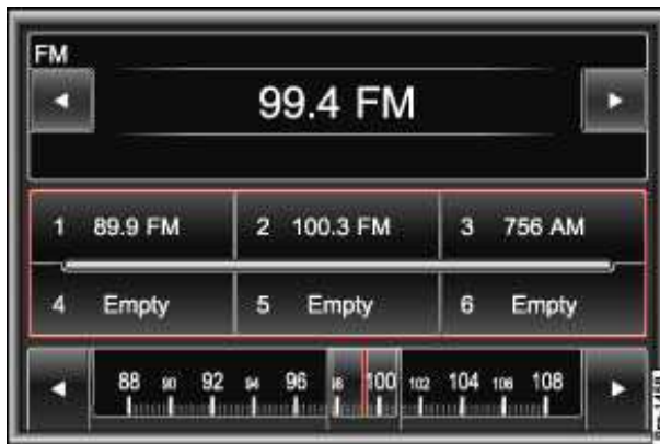
Fig. 137 RADIO main menu with the frequency dial for the selected frequency band.
