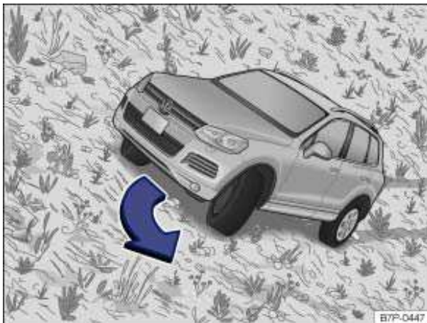
Fig. 283 Steer downhill along the fall line.
