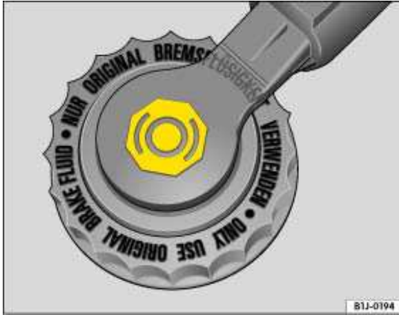
Fig. 248 In engine compartment: Brake fluid reservoir cap.
