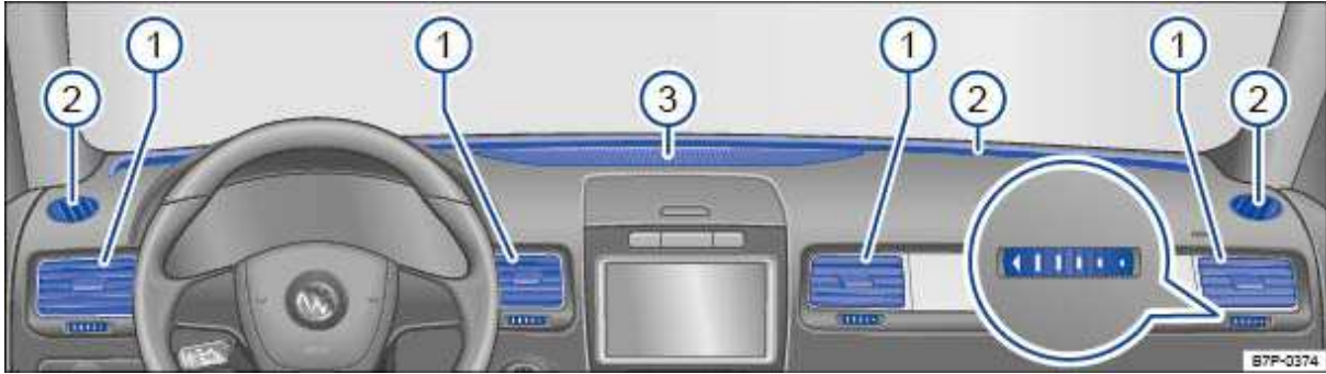
Fig. 274 Air vents in the dashboard.
