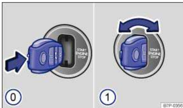
Fig. 241 In the ignition switch: Vehicle key positions.
