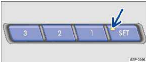
Fig. 55 Memory buttons in the upper part of the driver and front passenger doors.
