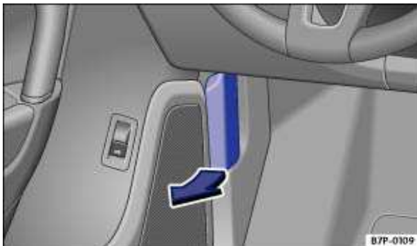
Fig. 285 Inside hood release lever in the footwell on the driver side.
