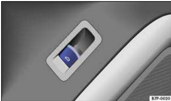
Fig. 28 In the driver door: Power button to unlock the rear hatch.
