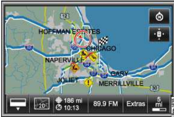
Fig. 214 SIRIUS traffic flow display and traffic congestion on the map.
