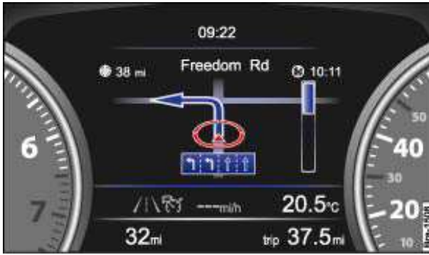
Fig. 211 Visual navigation recommendations in the instrument cluster.
