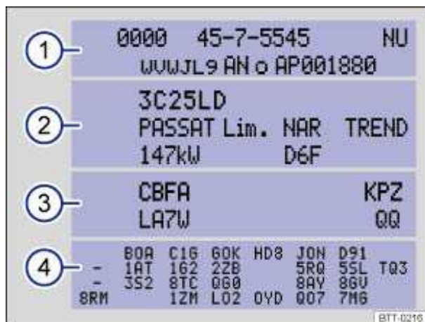
Fig. 15 Vehicle identification label: Shown in the example with engine identification code CBFA.
