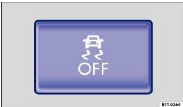
Fig. 247 In the front center console: Button to manually switch ASR on and off.
