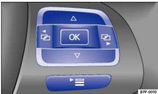
Fig. 14 Right side of the multi-function steering wheel: Controls for the menus in the instrument cluster.
