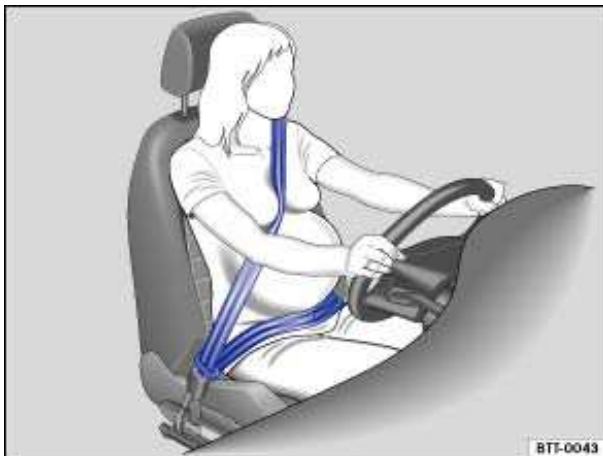
Fig. 66 Proper safety belt positioning for expectant mothers.
