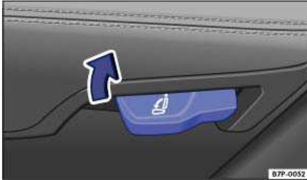
Fig. 98 Lower part of the rear seat bench: Lever to unlock the rear seat backrest by hand.
