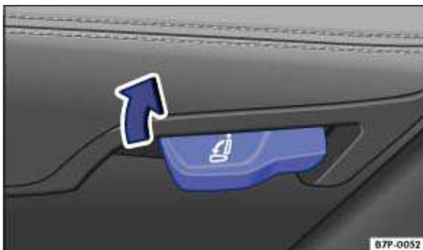
Fig. 44 Adjusting angle of left rear seat backrest.
