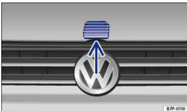
Fig. 286 Outside hood release in the radiator grille.
