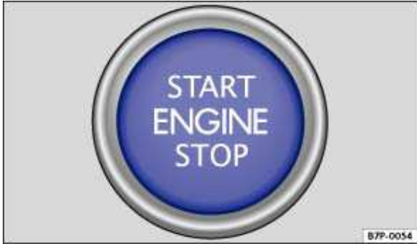
Fig. 242 In the front center console: Starter button of the Keyless Access locking and starting system.
