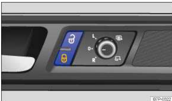
Fig. 24 On all 4 doors: Power locking switch.
