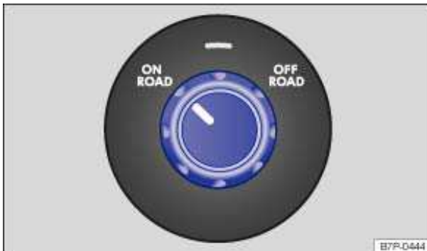
Fig. 282 In the lower front center console: Rotary knob (4MOTION).
