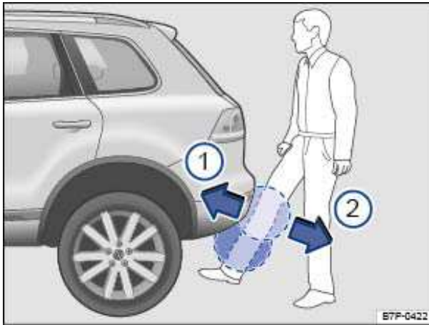
Fig. 26 Access locking and starting system: Opening the sensor-controlled rear hatch (Easy Open).
